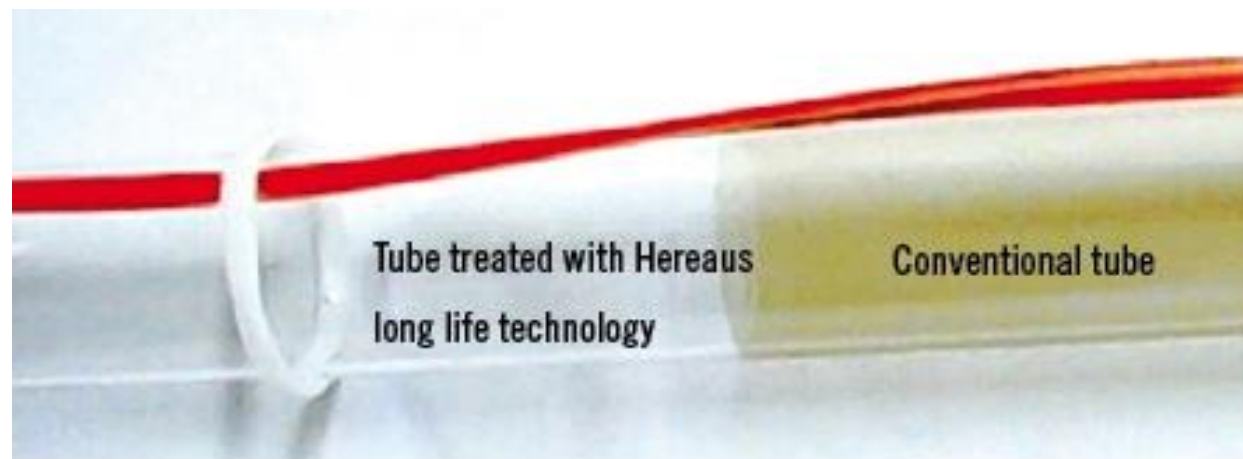
380 W lamp after 10,000 hours operation
