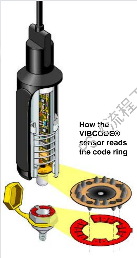
How the VIBCODE® sensor reads the code ring
