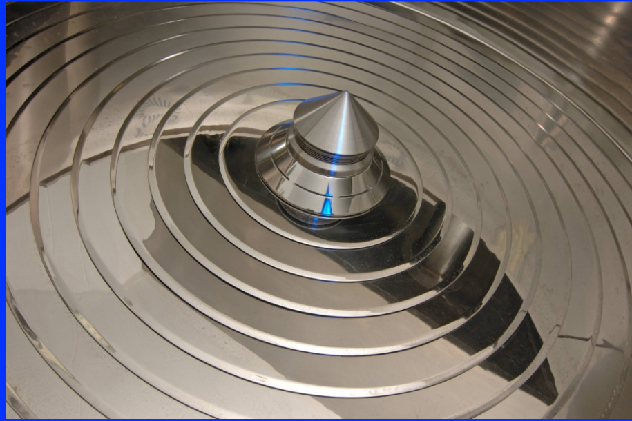
INNOJET Booster ORBITER center view with INNOJET spray nozzle ROTOJET
