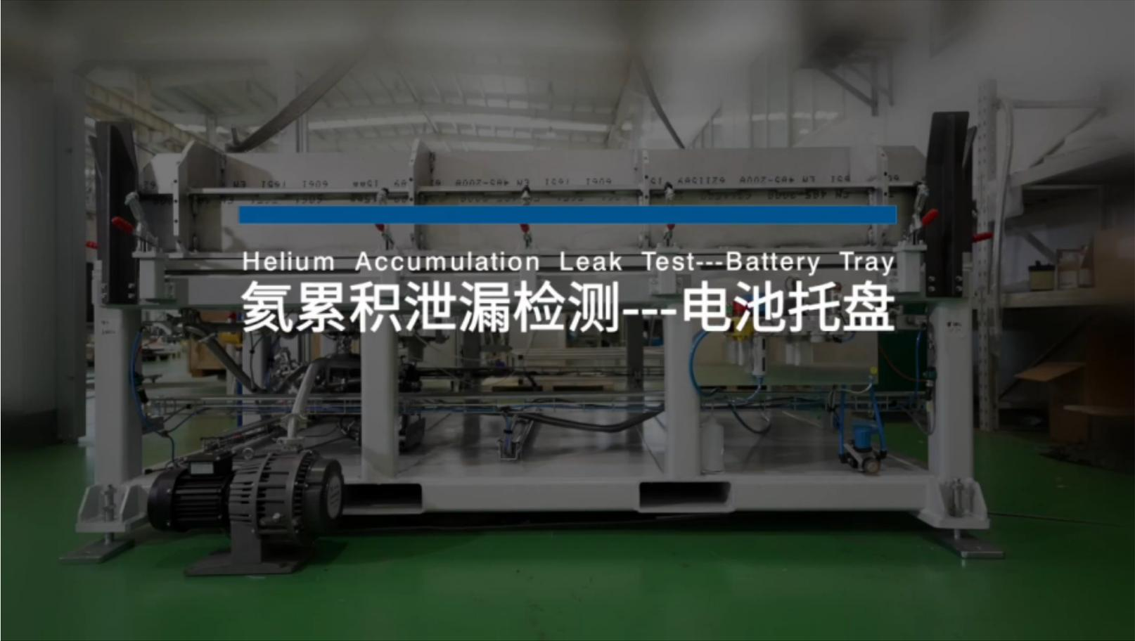
Helium Accumulation Leak Test---Battery Tray
