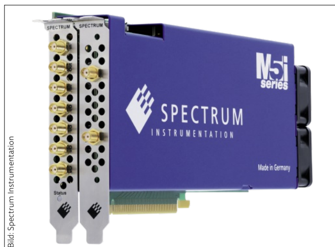
Two PCIe digitizer cards from Spectrum Instrumentation's M5i family feature a sampling rate of 10 GigaSamples per second.
