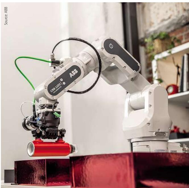
Swifti is a fast and precise collaborative industrial robot with a speed of 5 m/s and a payload of 4 kg.
