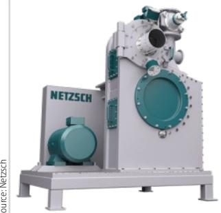
In the Secomy S, Netzsch has solved the classifier sieving problems in their standard fine-cutting mills in the range under 125 µm. Separation now works without a sieve, using a dynamic classifier wheel improved for fibrous products. Coarse material falls back into the grinding space. Fine particles leave the machine.
