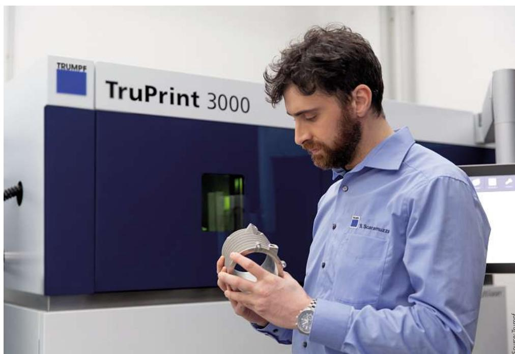
This medium-format machine uses powder-bed-based laser melting to produce components of up to 300 mm diameter and 400 mm height.
