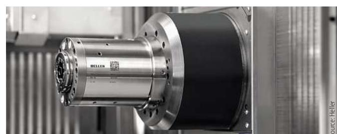
A central feature of the new HF series are the new machining work units.
