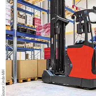
The rack-protection sensors initiate dynamic braking of the machine when an obstacle is detected.
