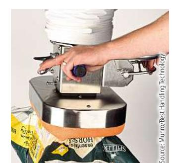
Rolls and coils, products with smooth surfaces, and also KLTs and cartons, can be moved using a vacuum lifter.
