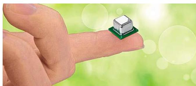
SSCD4x from Sensirion: these selective CO<sub>2</sub> sensors are extremely small.
