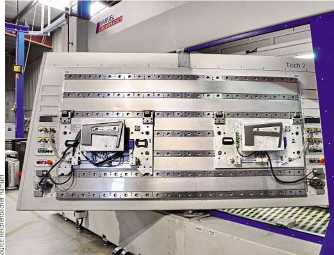
The ECO-RS-III creates, for example, aluminium trims for automobile interiors.
