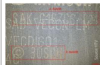
Renamed component: after the wipe test the original lettering reappears.
