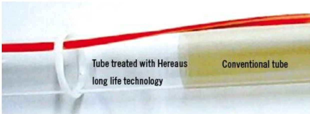
380 W lamp after 10,000 hours operation
